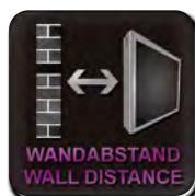
**wall distance** The value shown indicates the wall distance in millimeters. For extensible wall mounts, there is a value for minimum and maximum wall distance.
